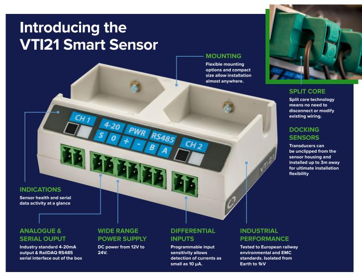
The VTI21 has been designed for the monitoring of railway assets that require high-speed sampling and/or multiple input channels. The VTI21 contains an on-board microprocessor that takes raw incoming waveforms and derives computed values that are most relevant from a condition based maintenance perspective. The VTI21 can derive many output parameters from the source waveforms and all of these parameters can be output over the RS485 data link to a connected MPEC data logger.
